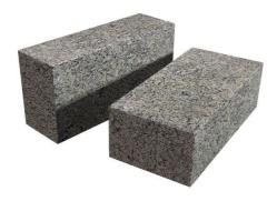
The BBX block system is similar to concrete blocks, composed of cement and fine aggregates, but with a difference, using bespoke materials instead of stone aggregate as part of the mix. This material provides the block with substantial tensile capacity and
